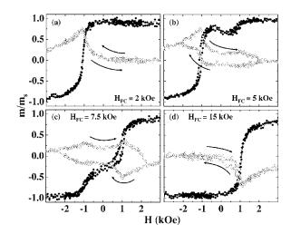
FIG. 1. Longitudinal ( $m_{\parallel}$ , solid circles) and transverse ( $m_{\perp}$ , open circles) magnetic hysteresis loops of Ni/FeF<sub>2</sub> field cooled in  $H_{FC}$  of (a) 2, (b) 5, (c) 7.5, and (d) 15 kOe. The moments are normalized to the saturation moment  $m_s$ . Arrows indicate the field-cycle sequence for the transverse loop.
